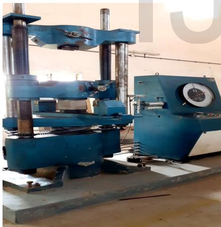
Fig. 1 Testing of cube in universal testing machine
